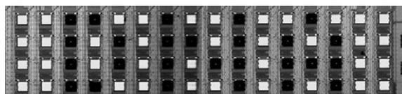
**Fig. 10** The FBAR array with some of the pixels functionalized. The black squares are drops of liquid containing probes and Lipa-DEA. The squares appearing in white are uncovered gold pixels.<sup>50</sup> Reproduction of the figure has been made with permission from the Molecular Diversity Preservation International.
